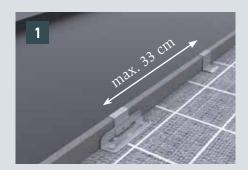
In the modular panel area (see fig. 7) the maximum 33 cm distance between clamps (centre to centre) must not be exceeded.
