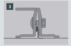
The installation direction of the bracket should be selected so that the threaded rod can then be mounted on the fold side.
